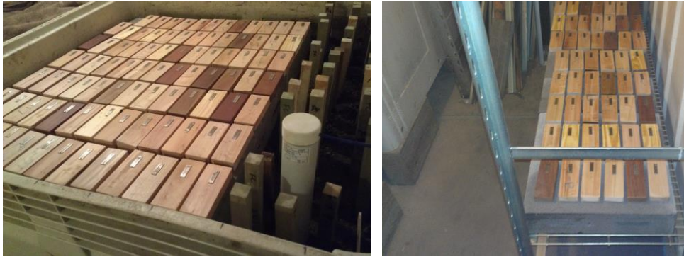
Figure 2 Modified ground proximity tests at Salisbury Research Facility (left – SRF on soil, right – SRF on shelf)
