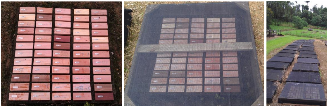
Figure 1 Ground Proximity field test at South Johnstone research facility
