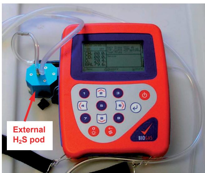
Figure 8. Geotech Biogas Check portable gas analyser used to monitor biogas quality.
