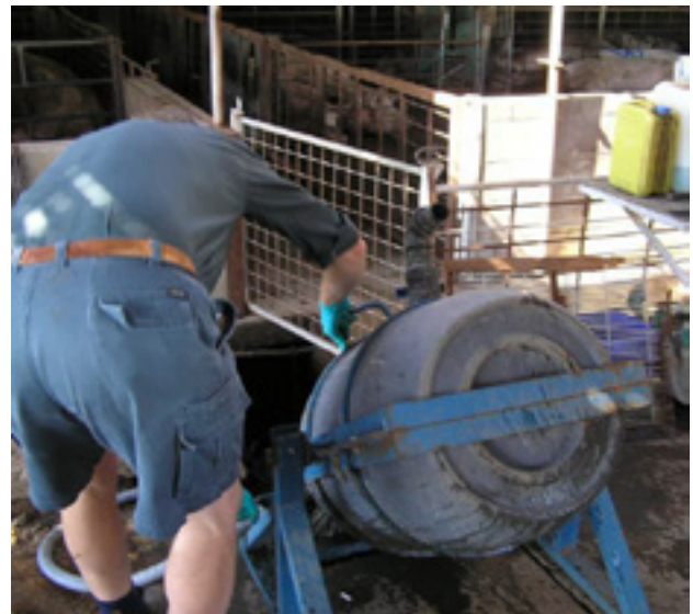
Figure 15. Tipping drum contents into sump after sub-sample collection.
