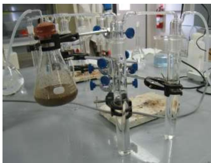
Figure 6. The ammonia headspace apparatus in use for technique development. Two impingers, filled with 50 ml of 0.25 M sulphuric acid are connected to the ammonia source, with a constant flow of air from the source through the impingers.
