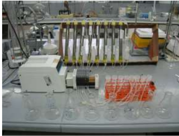
Figure 4. Leaching in-progress using a multi-channel peristaltic pump.
