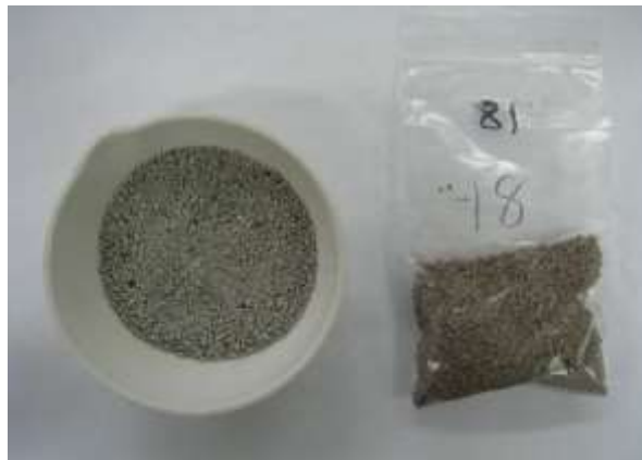
Figure 2. Bentonite was ground and sieved to between 0.5 to 2 mm (left). An example of the pelletised litter fertiliser with bentonite and hydrotalcite is on the right. All experimentation was conducted with 0.5 to 2mm pellets.
