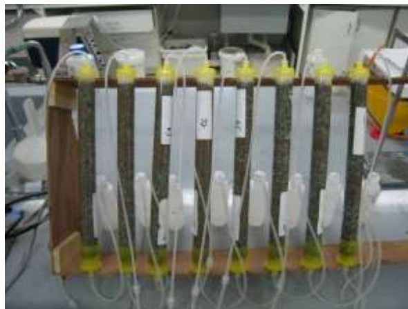
Figure 3. Columns prepared for the leaching trial. Note the 3:1 volume ratio of polyethylene beads to pelletised litter treatments. The admixture of beads prevents blockage and allows effective daily drainage to prevent development of anaerobic conditions.
