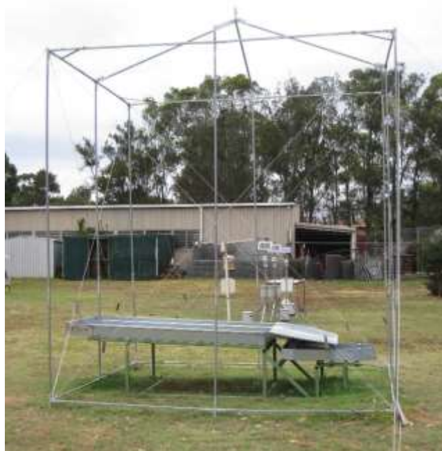
Figure 5. Rainfall simulator assembled over a the dual flume apparatus.
