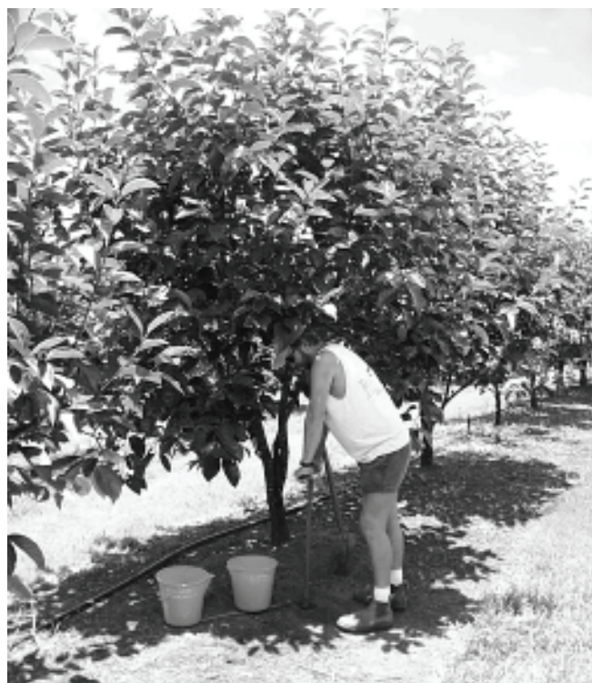
Figure 23 (a). Select a sampling site under the tree canopy within the wet area from the sprinkler
