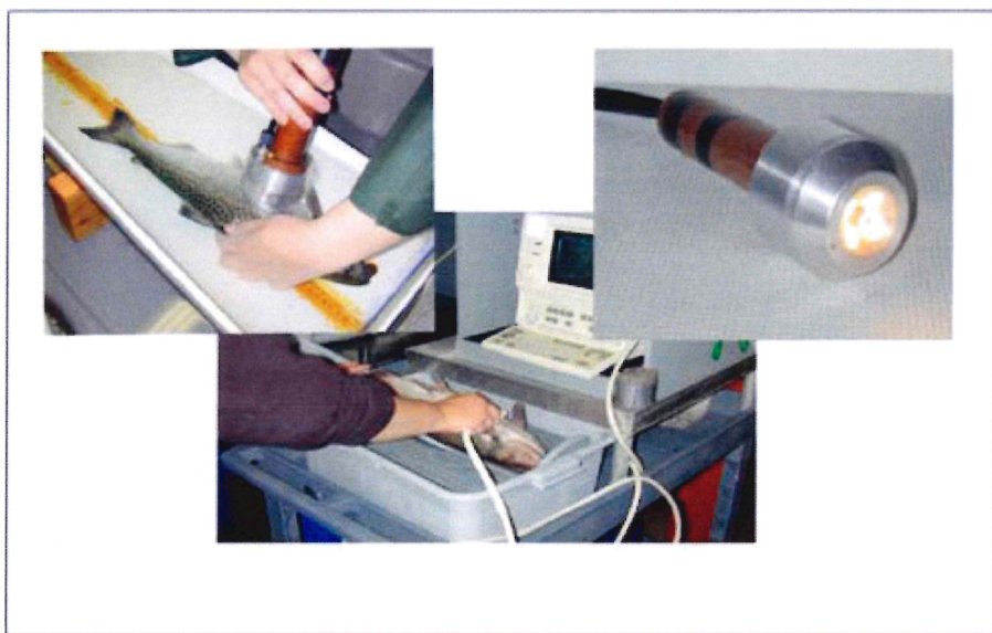
Figure 28. An image from Davis et al (2006) showing the use of the SW-NIRS device on a Chinook salmon.
