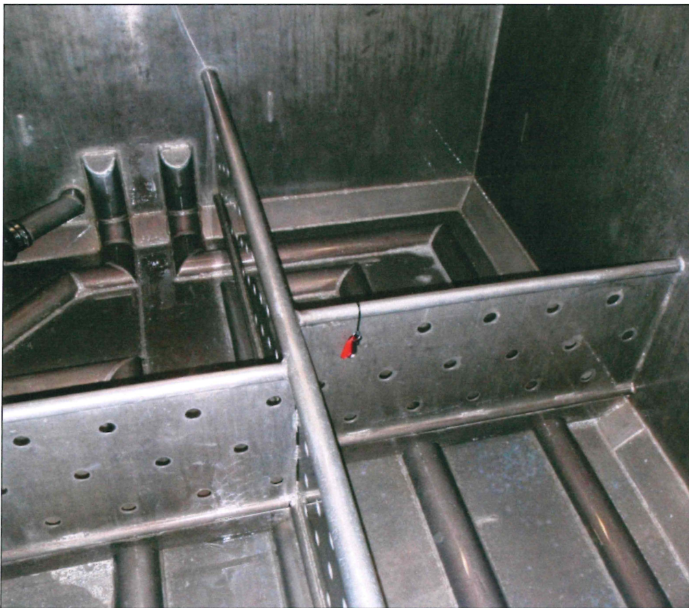
Figure 5. Temperature logger in brine tank (red tag).
