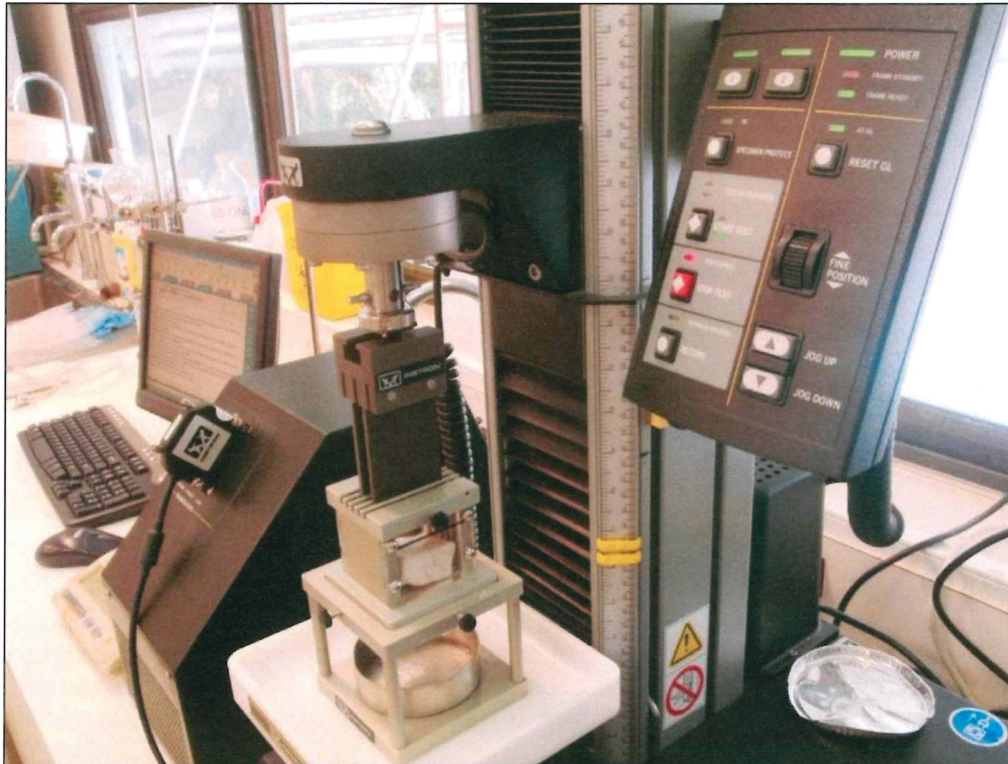
Figure 2. Instron texture analyser with sample loaded into the Kramer-Shear cell.
