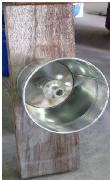
Figure 13. The ejector mounted inside a metal bucket and attached to a backboard
