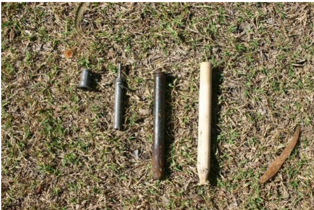
Figure 6. Components of a cyanide ejector and wooden stake as used in the pilot trial
