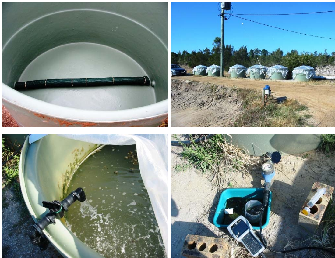
Figure 2 Experimental polychaete sand beds at the Bullock Creek Prawn Farm including the tank drainage system before filling with sand (top left), the positioning of tanks with covers on pond embankment (top right), the inside of a tank during operation (bottom left), and a tank's drainage water meter and collecting tub for sampling (bottom right).
