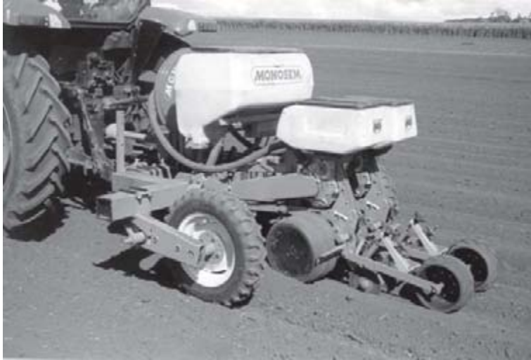
Figure 12. Side and rear views of a two-row planter also applying basal fertiliser and laying drip tape
