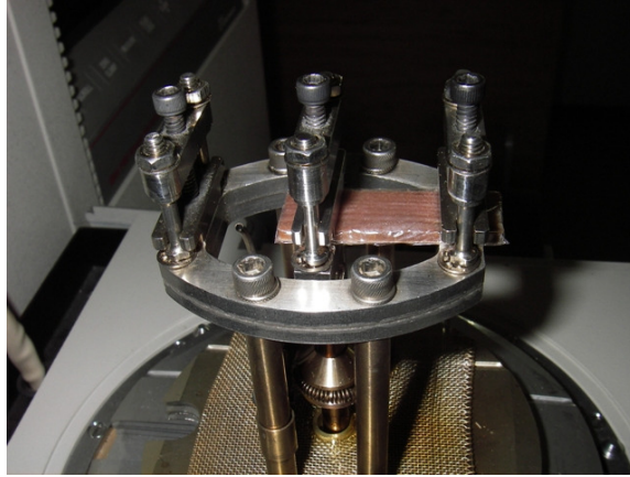
Plate 8. Sample wrapped in plastic film and placed in clamp for DMA testing
