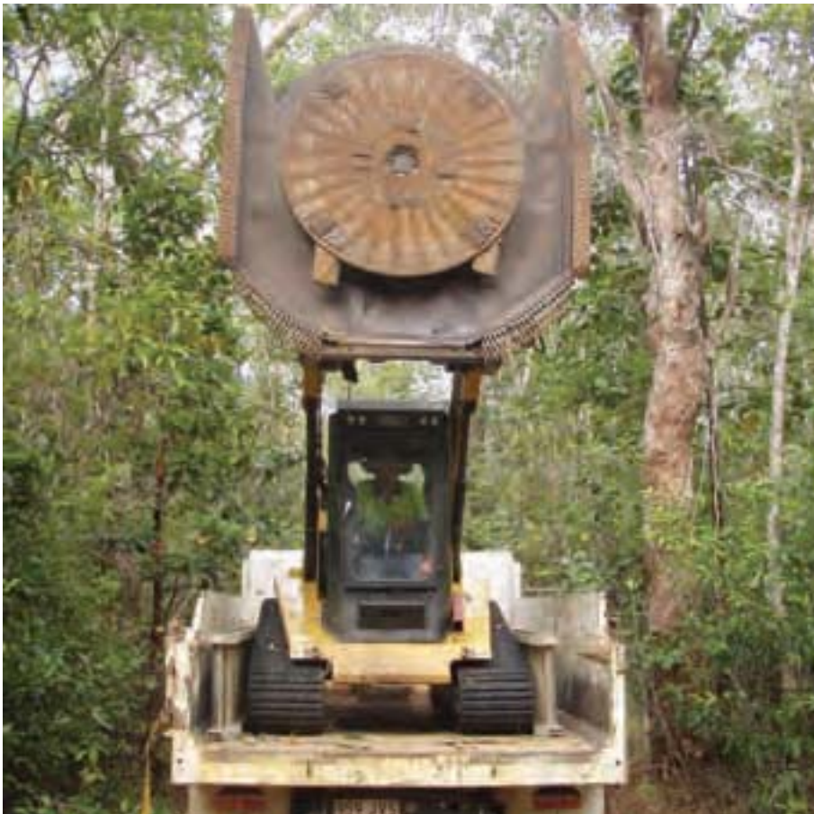
Photo 1. The Positrack is a tracked bobcat with a robust slasher-type attachment that cuts individual trees off near ground level and reduces them to mulch.
