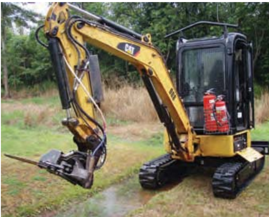
Photo 2. The Tracksaw is a tracked mini-excavator with a chainsaw bar and spray applicator on the boom that cuts individual trees off near ground level and applies chemical immediately to the cut stump.
