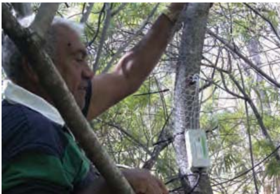
Photo 2. Dr Faiz Bebawi inspecting a sap flow sensor installed on a Captain Cook tree.
