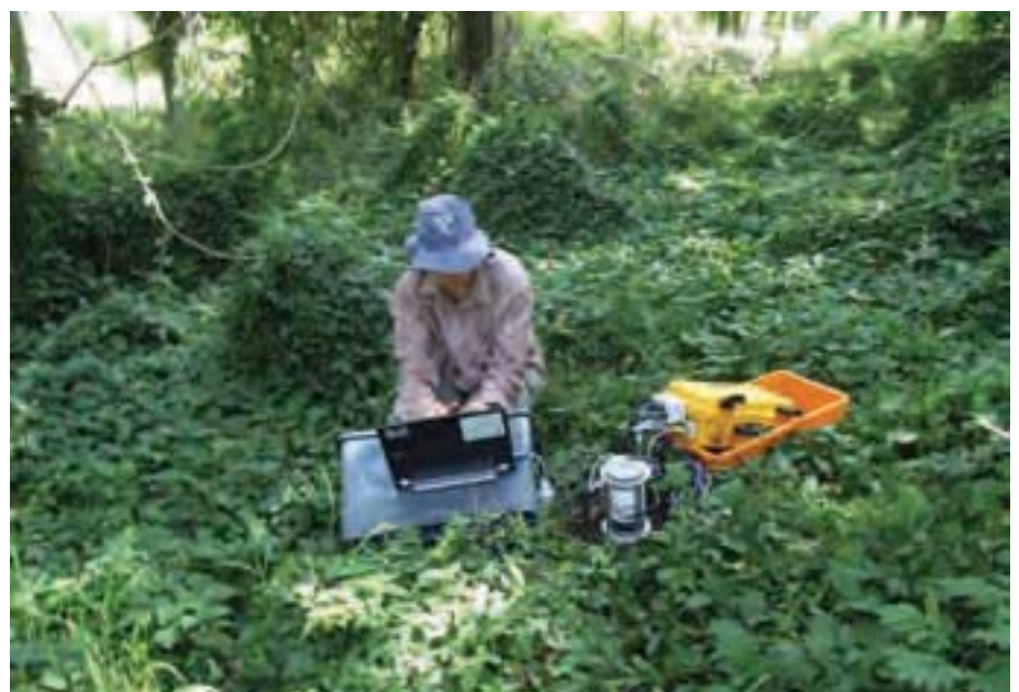
Photo 1. Experimentalist Christine Perrett undertaking soil respiration measurements in a cat's claw creeper-infested landscape.
