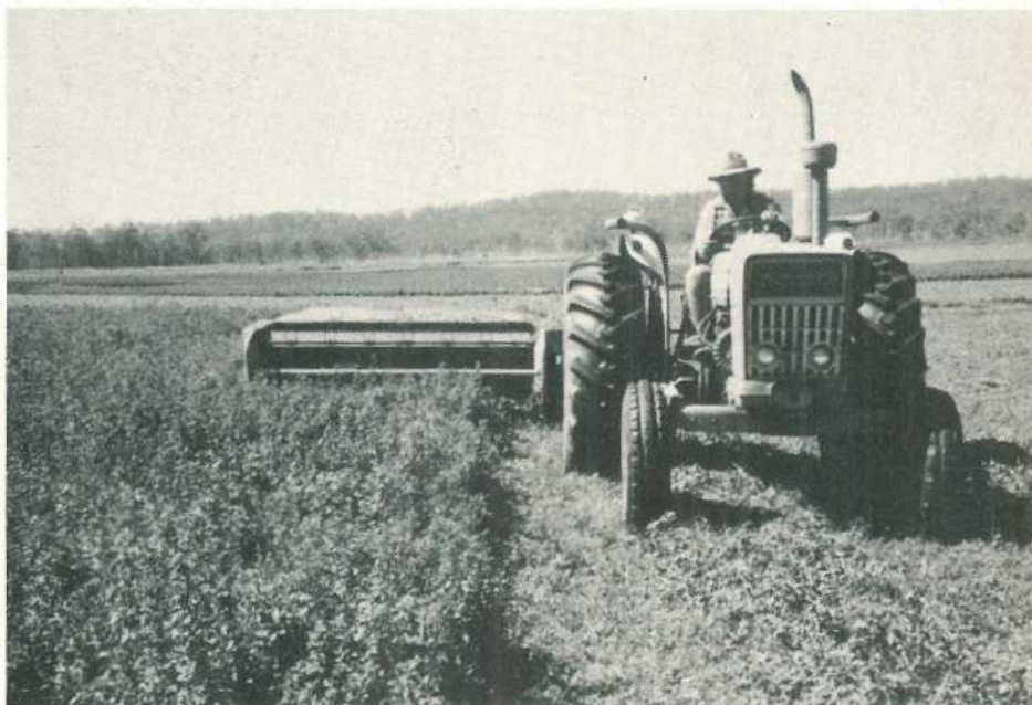
The haybine mows, conditions and windrows.
