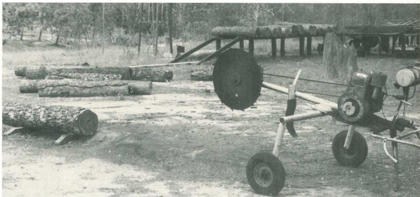
A flitch is cut from one side of each ironwood log with a hargen saw before the log goes on to the saw bench.
