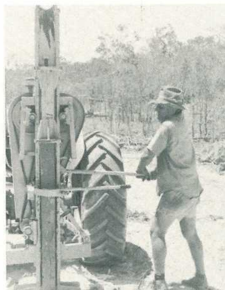
John Harris uses a friction-drive tractor-mounted post driver.
