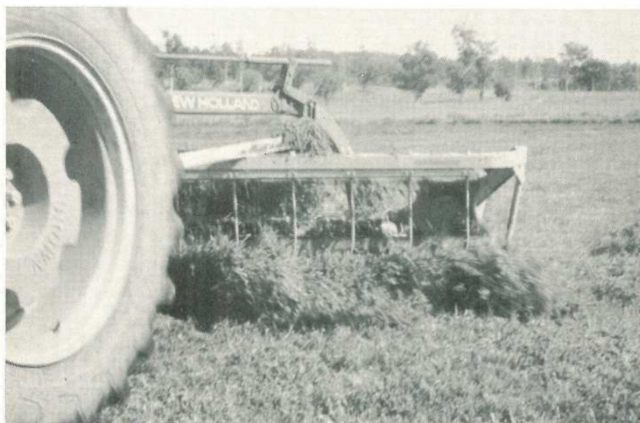
The side delivery rake is still widely used to turn windrows and ensure quick and even drying prior to baling.
