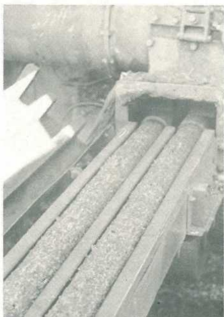
The dried, compressed lucerne coming out of a wafer machine. This machine makes about 1 t per hour of wafers.
