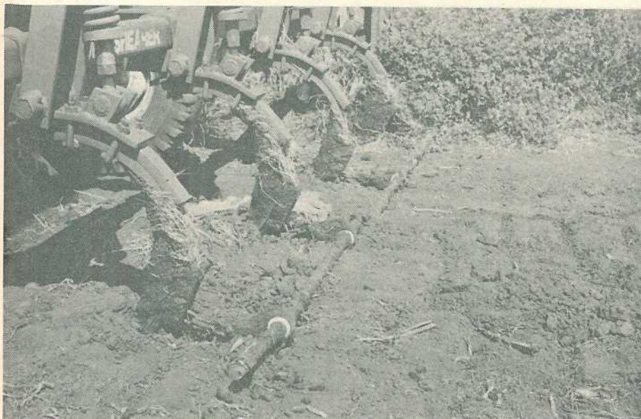
Rod-weeders are a useful addition to the chisel plough. They give good weed control while the chisel plough works at depth.
