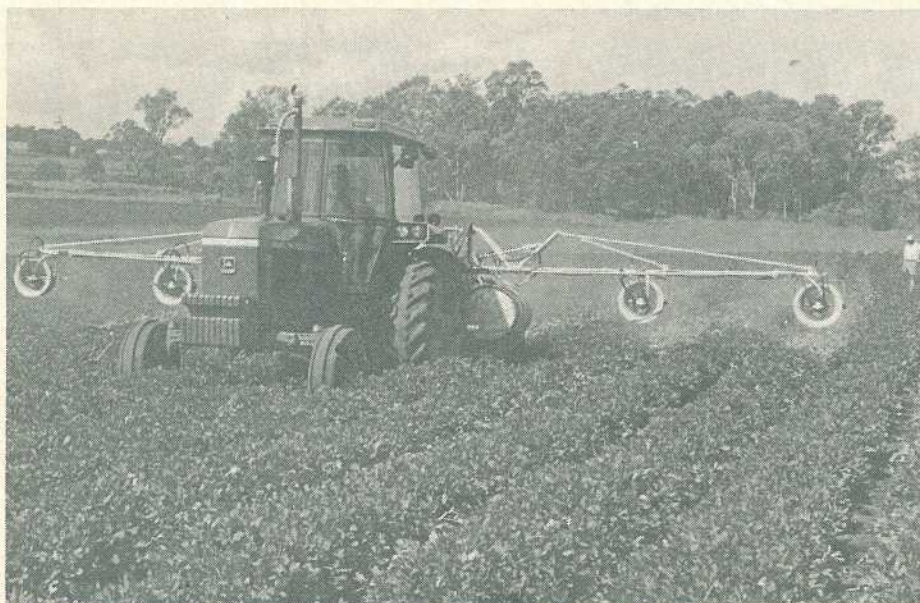
Ground-operated 'Micronair' spray rig. This recently-introduced equipment precisely controls pesticide application.
