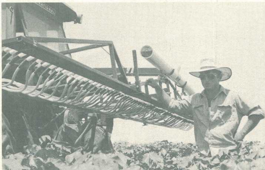
Rope wick applicators are being used to control tall-growing weeds in cotton and soybeans.
