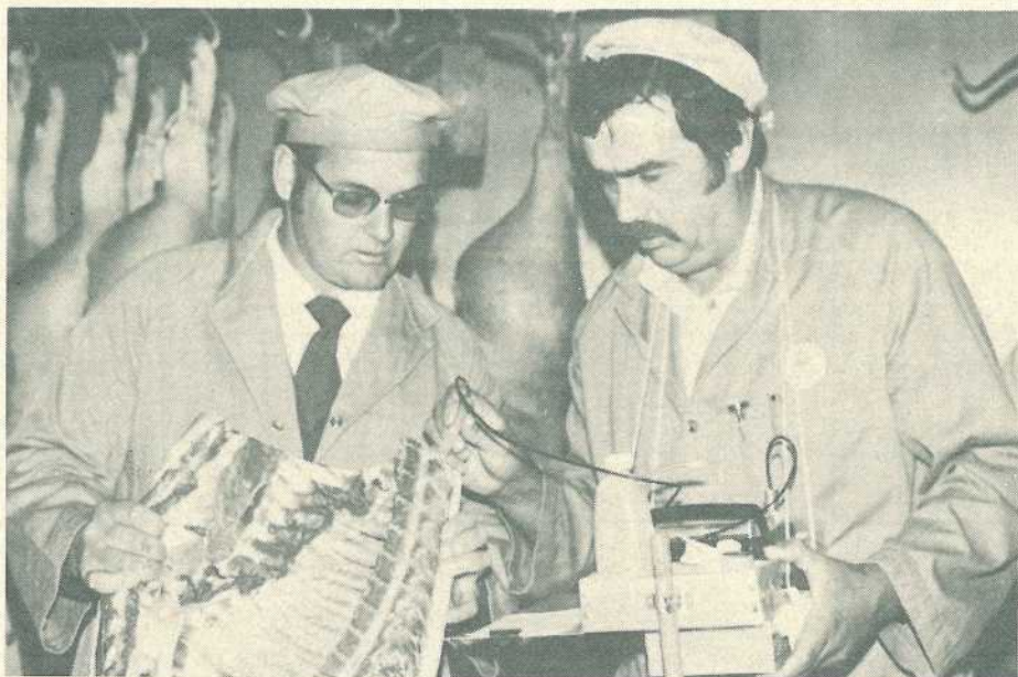
Stewards using a pH meter as an aid in determining colour score.
