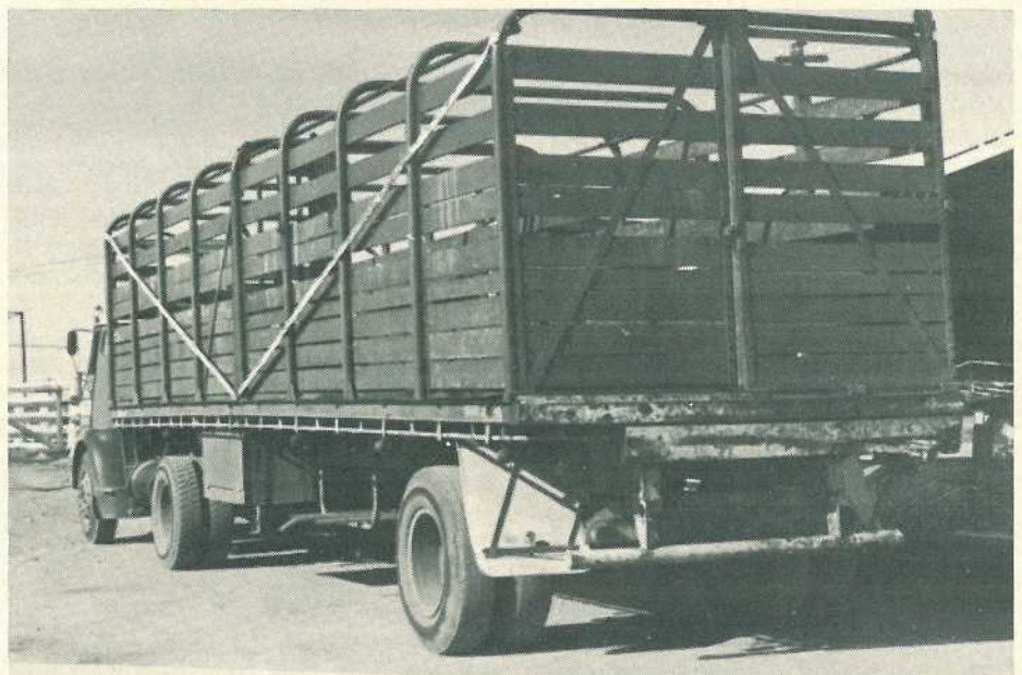
External structural supports ensure a smooth lining. A non-slip floor also helps reduce the risk of bruising.
