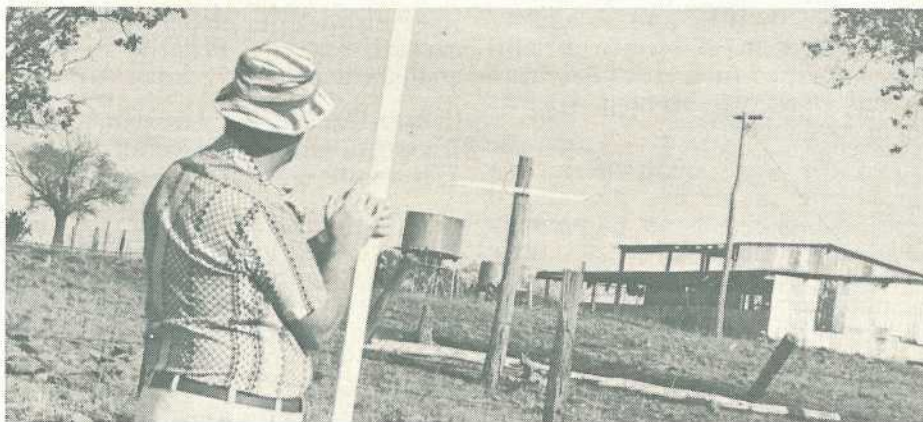
Plate 1. Reasonably accurate measurements can be taken of a water level in a tank by using a graduated scale and a sight mark attached to a dead tree, wall or fence post.
