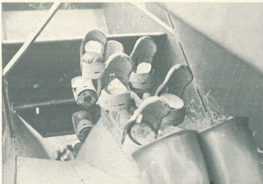
Cup type potato planters use holders to separate individual setts for uniform plant spacing. A double row planter is illustrated.
