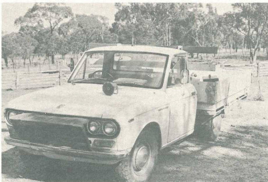
This mobile station has a speaker mounted on the bonnet. The driver can be called up at a distance of 150 m from his vehicle.
