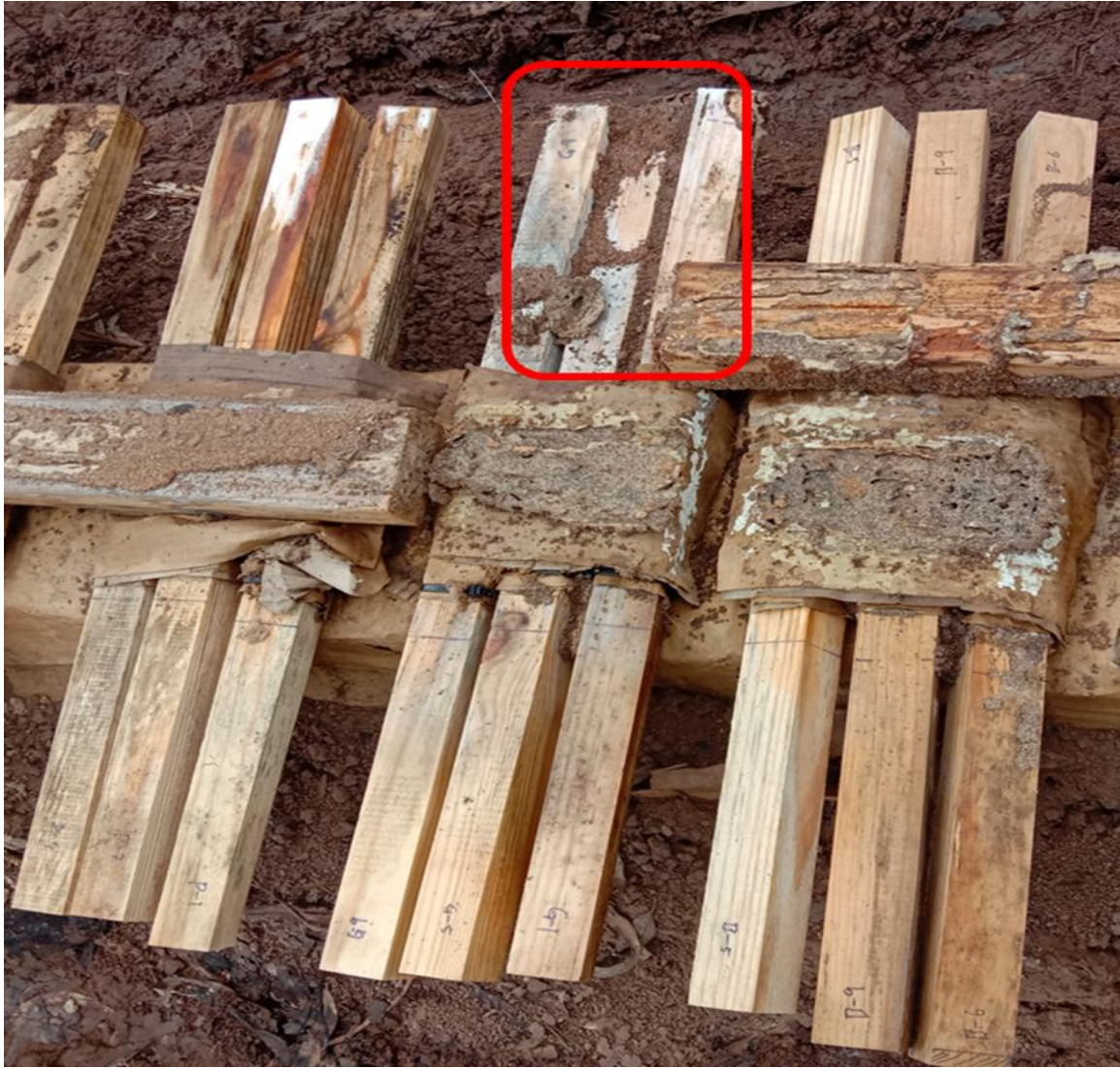
Figure 5: Example of termite behaviour where soil transport and surface sealing outside the central exposure zone enabled attack to extend along the beam length, resulting in extensive damage outside the flexure zone.
