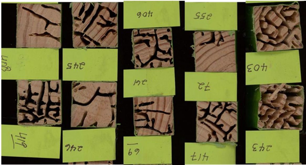
Figure 9: Example of transverse cross-sections of pine beams after subterranean termite exposure, showing varying degrees of internal damage and loss of effective cross-sectional area
