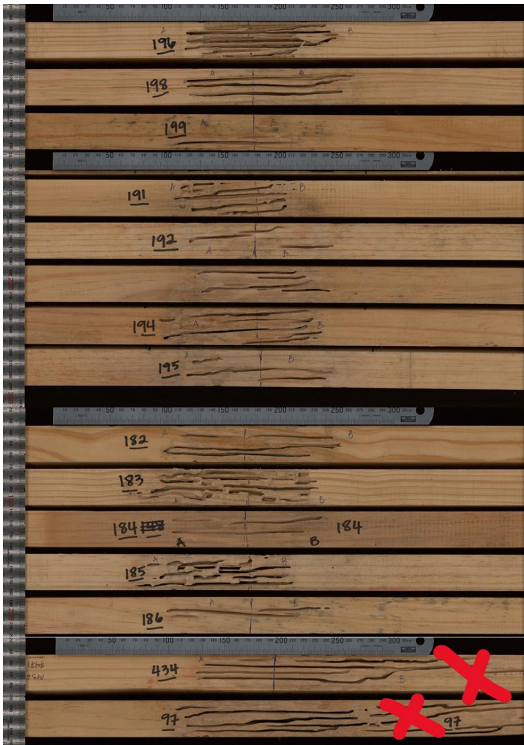
Figure 4: Examples of pine beams after subterranean termite exposure, showing predominantly localised damage within the designated central exposure zone. In most specimens, termite galleries were confined to the beam centre. Beams marked with an “X” experienced damage extending beyond this region and were excluded from post-exposure testing.
