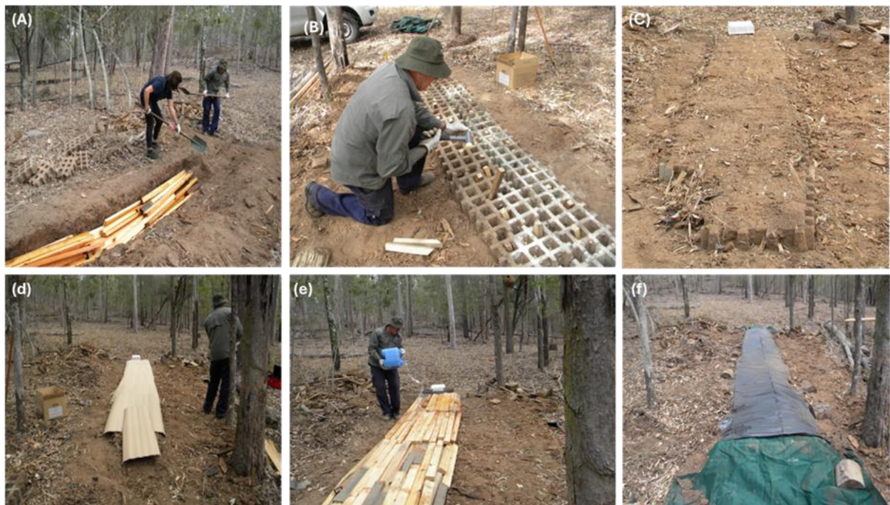
Figure 2: Steps used to prepare a trench for termite testing: Trench being filled with feeder wood (a), concrete blocks with stakes to encourage upward termite movement (b), blocks covered with soil (c) and then corrugated carboard (d), final assembly with pine feeder material on top being wetted (e) and then the covering tarp to protect the termites (f).
