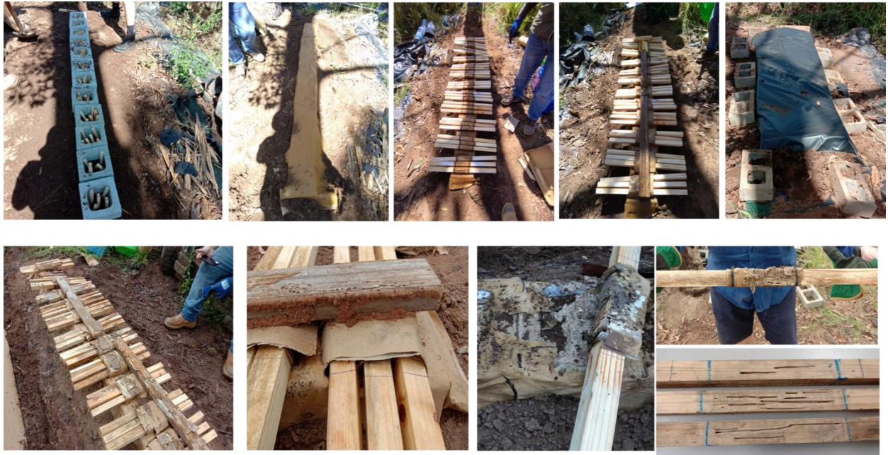
Figure 3: Field exposure setup showing timber beams positioned on hollow concrete blocks to encourage termite attack in the central portion of the beams (top row). Preliminary trial demonstrating that, in most beams, termite attack was successfully restricted to the designated central exposure zone (bottom row).
