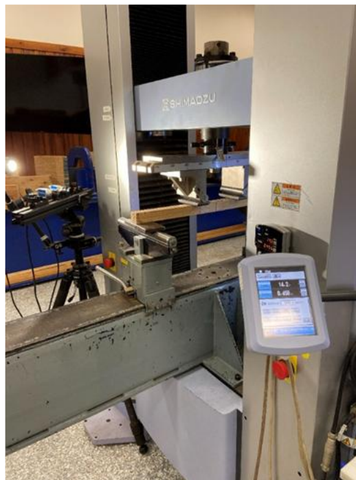
Figure 1: Four-point bending test of a timber specimen using a Shimadzu universal testing machine.
