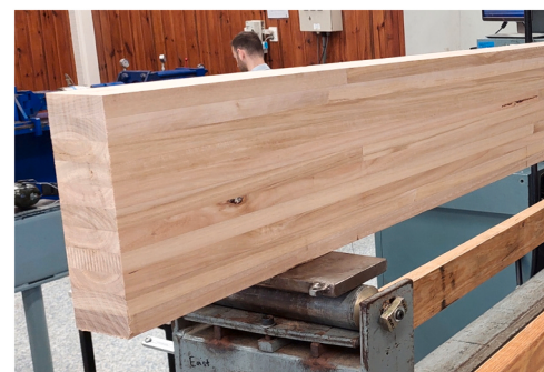
Fig. 8. Example of a GLT beam manufactured and tested in Gilbert, et al. [84].
