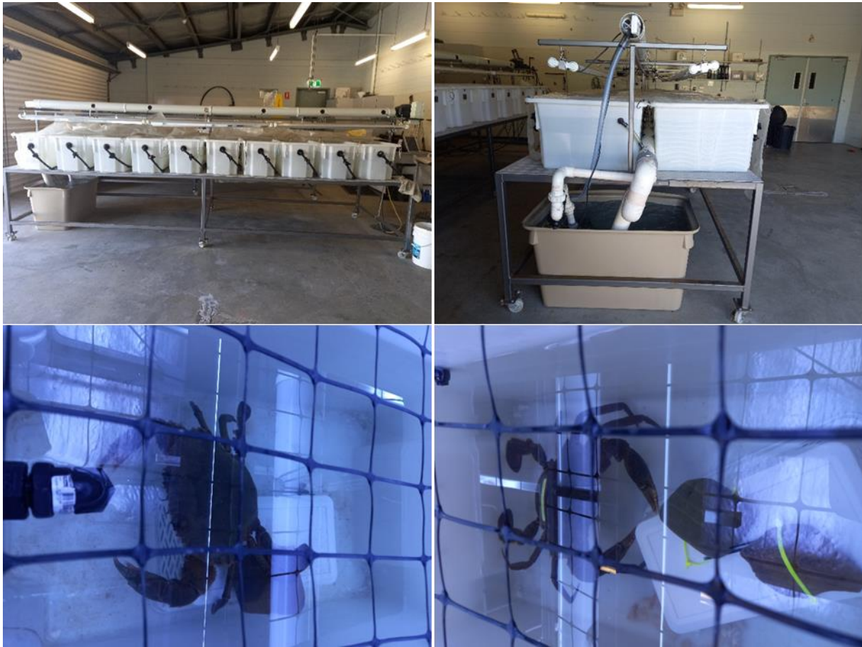
Figure 24. Recirculating seawater system housing Giant Mud Crabs in individual tanks for Tagging Experiment 2: mortality and moult retention (individuals in 50-L tanks).
