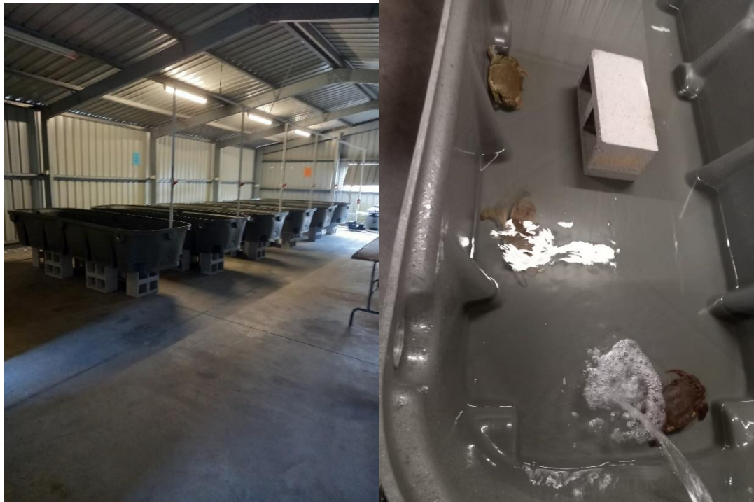
Figure 25. Purpose-built recirculating seawater system at CQUniversity's Gladstone campus, housing crabs in groups of three. Lids were added to the tanks one week after crabs were introduced, and then the water level in troughs was increased to approximately 40 cm.
