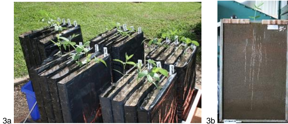
Figure 3a: Twenty 600 x 400 x 50 mm root chambers positioned into five randomised replicates (photographed on 13th January 2021 at day 23).
