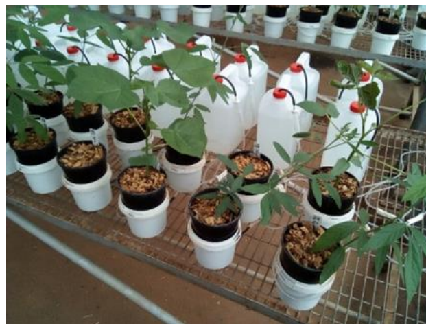
Figure 2: Pot-in-bucket lysimeter. Plants were grown in 150mm pots positioned in buckets with a constant water table. The water table was regulated with a float valve in the bucket and fed using a syphon from the 5 L water reservoir. To minimise pot evaporation, the soil surface was mulched with 25mm of pine wood chips. Water used from the reservoir was quantified by weight.
