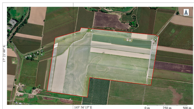
Fig. 1. High resolution RGB (Red, Green, Blue - visible spectrum) drone orthomosaic image reveals the location of palaeochannels close to ground surface. The drone image (outlined with a red line and in lighter shade) is superimposed onto satellite imagery obtained from the Global Mapper software (Source: Marcus Bulstrode, Queensland Government Department of Primary Industries).
