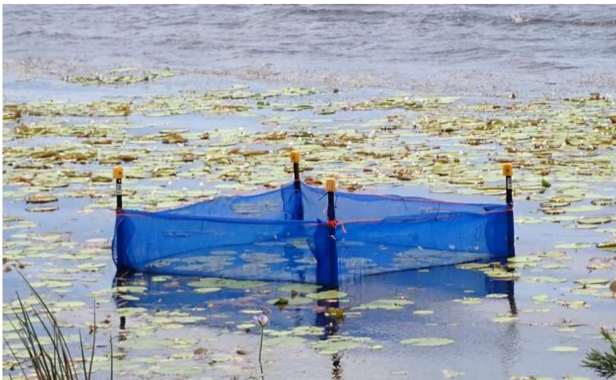
Figure 2 An enclosure installed in a lake to test the effect of cabomba removal with flumioxazin on the regeneration of native aquatic plants from the seed bank.
