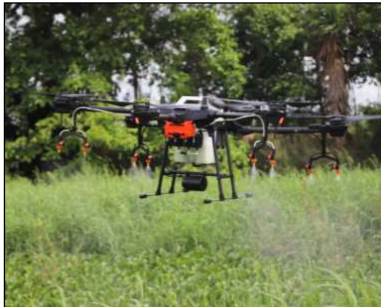
Figure 40 The Aleman grass herbicide trial site was sprayed using a DJI Agras T16 spray drone.
