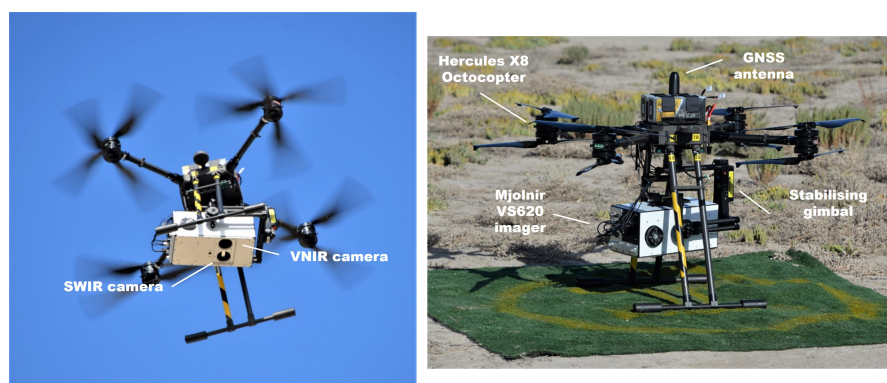
Figure 2. UAV hyperspectral imaging system showing the Blacksquare X8 Hercules multi-copter with mounted Hypspx Mjølfnir VS620 sensor.
