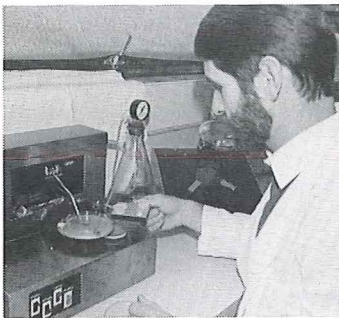
A spiral plating machine is used in a DPI laboratory to evaluate the bacterial count in a milk sample.
