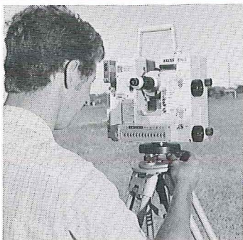
Electronic distance measuring equipment has boosted the collection rate of topographic survey data for soil conservation planning. The instrument computes and stores the co-ordinates of the height of a chosen point. These can be used to compose a computer-plotted map showing spot heights and contours.
