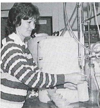
An officer in the DPI's agricultural chemistry branch dispenses an acidic extracting solution used in testing soils for available phosphorus, an important test for primary producers' soils.
