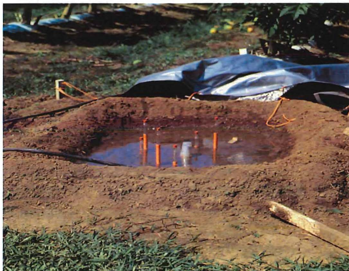
Photograph 1: Flooded bund at SJRS site, showing tensiometers and NMM tube.
