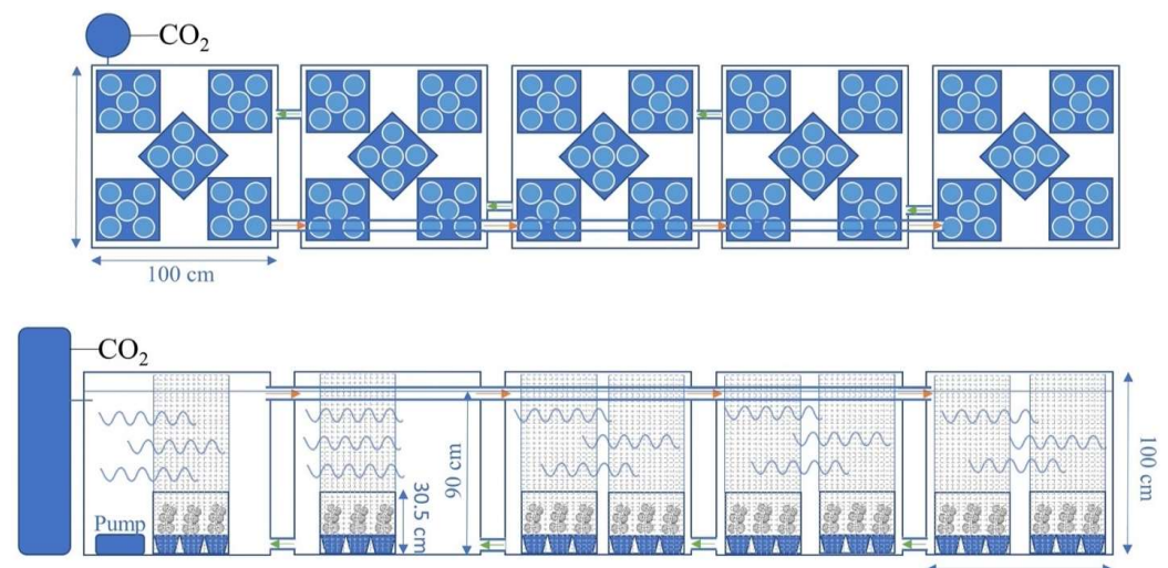
Figure 2. Schematic diagrams of the top and side views of the pond system used to culture cabomba before and after treatment in the regeneration experiment: Five ponds were interconnected with pipes to allow water to circulate between the ponds. The arrows indicate the direction of the circulating flow of the water. Each pond had five crates (blue squares) containing five pots with cabomba. Each crate was surrounded by a 30% generic plastic shade cloth held in place with four 100 cm bamboo stakes that reached above the water surface. The dimensions of the ponds and crates and the depth of water in the pond system are labeled. The pump that circulates water from the first to the last pond is shown in the first pond (from left to right), and a carbon dioxide injection device is connected to the first pond on the left.
