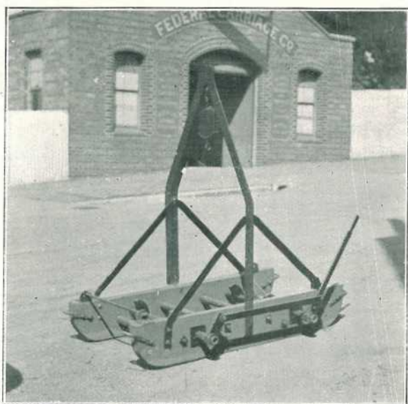
PLATE 95 (Fig. 1). Forster's Weight-grading Machine for Bacon or Pork Pigs, showing Construction of Framework.
