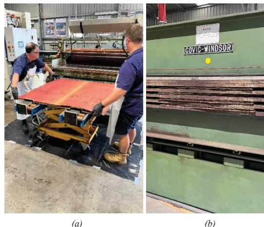
Figure 4. Selected stages of the LVL manufacturing (a) applying adhesive with a double roller glue spreader and (b) LVL being hot-pressed.
