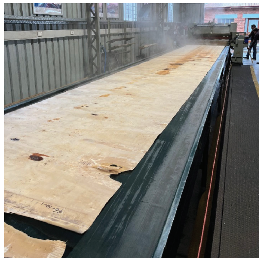
Figure 2. Veneer ribbon obtained after peeling.
