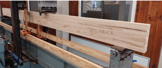
Figure 5. GLT beam tested in four-point bending.
