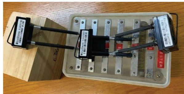
Figure 1: Sensor set up used for moisture monitoring.
