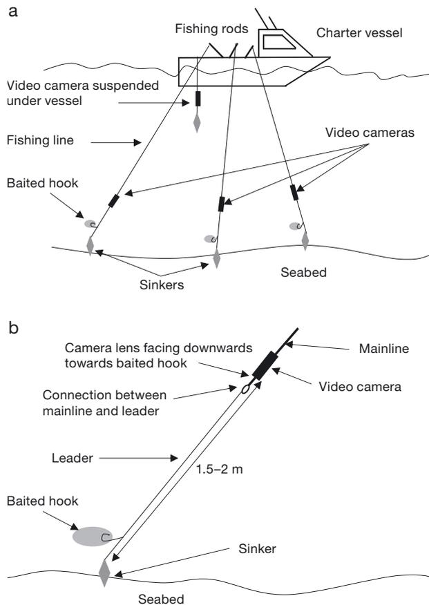
Fig. 2. (a) Video camera deployment on fishing lines close to the seabed and under the fishing vessel. (b) Close-up of the proximity of the video camera to the key components of the fishing gear, such as the baited hook and sinker. Diagrams not to scale
