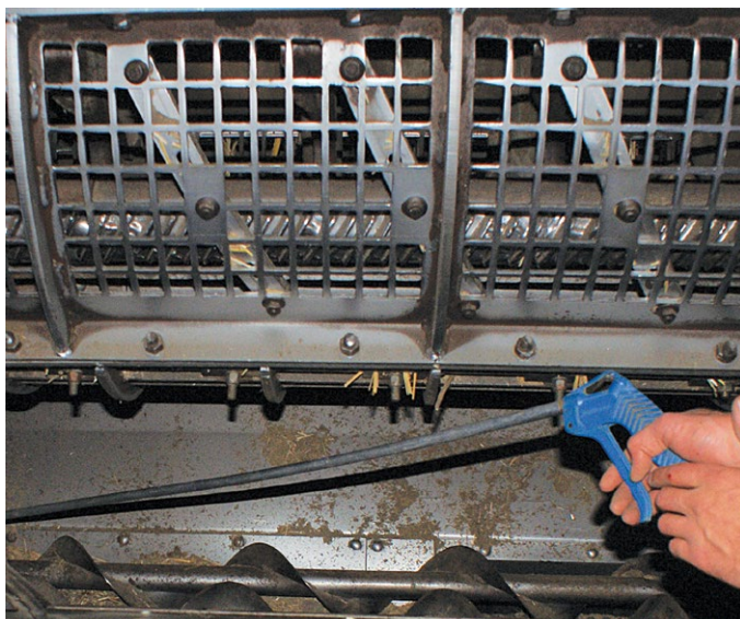
Clean out harvesters and grain-handling equipment thoroughly with pressurised air. Photo: Chris Warrick, Primary Business
