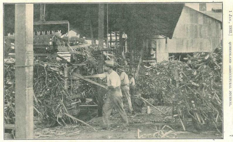
PLATE 1,-FEEDING CANE TO THE CARRIER, SOUTH JOHNSTONE SUGAR MILL.
