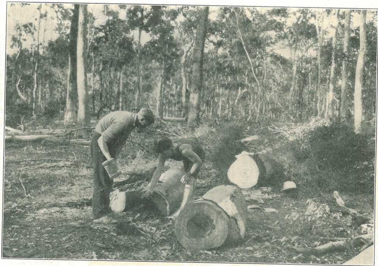
PLATE 37.—ENTERING A WEDGE. St. Lucia Trainees engaged in splitting fencing timber.
