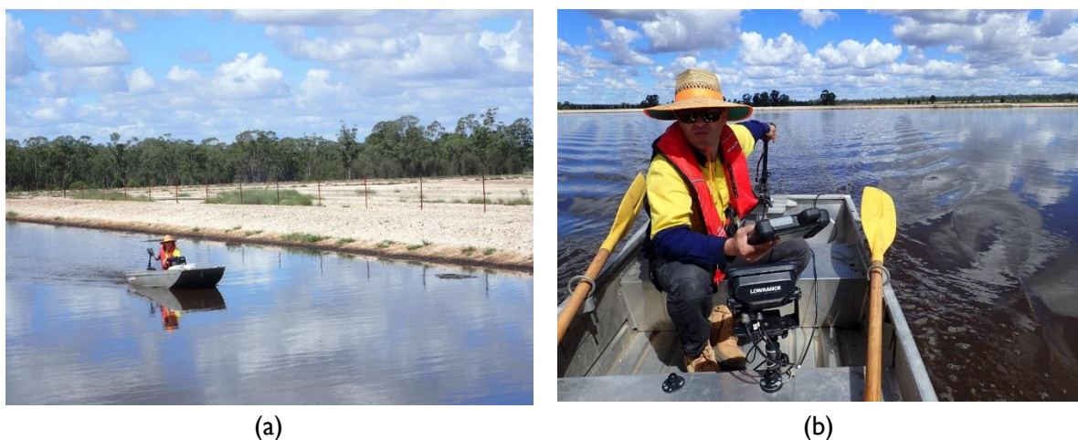
Figure 1 Premise Agriculture employee carrying out the hydro-survey to determine sludge profiles in secondary pond 4 at piggery A on 4 April 2017.
