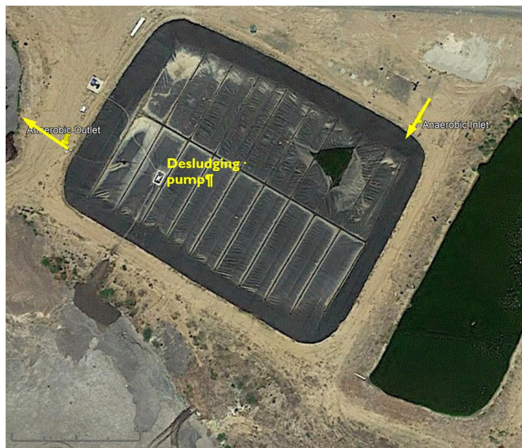
Figure 4 Aerial photograph (Google Earth) showing the effluent inlet and outlet and sludge sampling locations on the covered anaerobic pond operating at a large commercial piggery in southern New South Wales.
