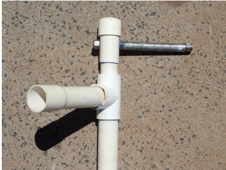
Figure B3 Sampling pole handles used to open and close the slot.
