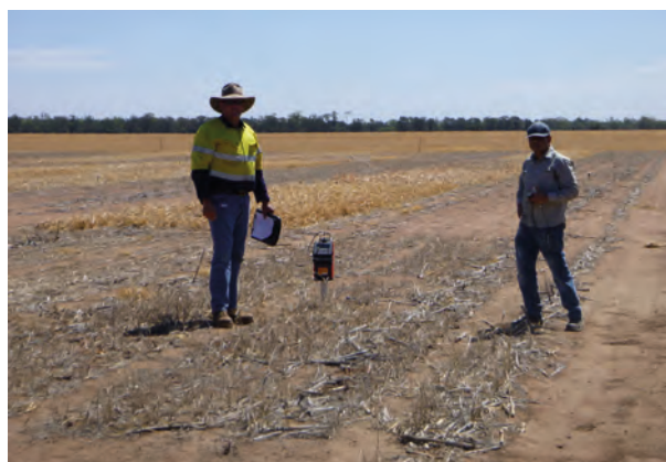
Taking monthly neutron moisture meter readings.
