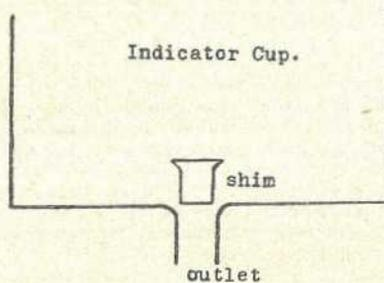
similar to that used to seal certain types of tobacco tins and should be fashioned in the manner indicated in the diagram. One or more may be tried, and should the result justify the opinion that the outlet is too large, steps should be taken to permanently reduce the size.
