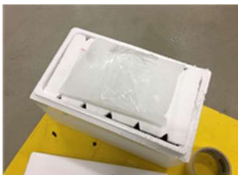
Image 9. Packout box configuration and partially thawed gelpack after 24 hours
