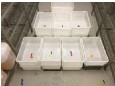
Image 12. Placement of bins with different insulation in cold room
