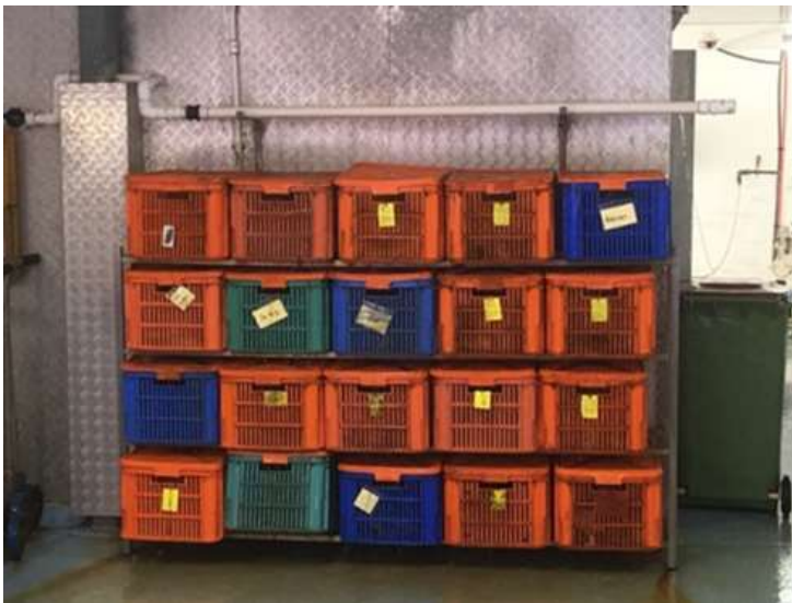
Image 11. Simple manifold drip system to hold crab cool and moist prior to transport
