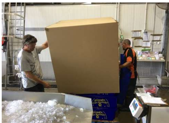
Image 10. Cardboard sleeve covering bins for insulation
