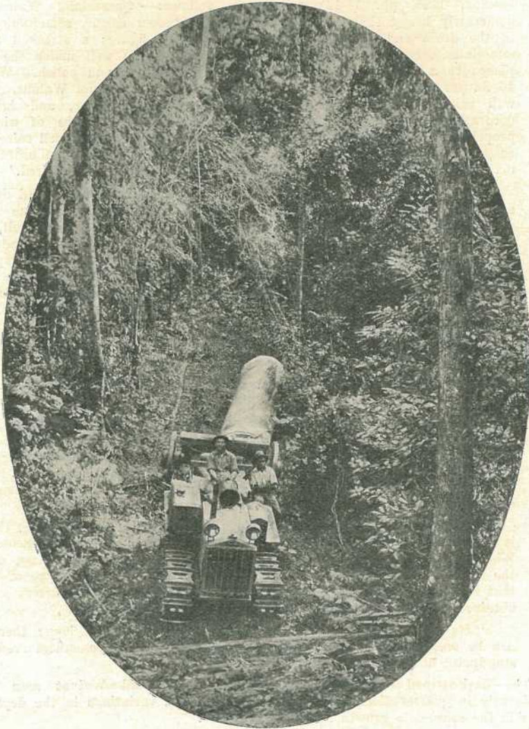
PLATE 47.—SNIGGING VENEER LOGS WITH TRACTOR IN A NORTH QUEENSLAND FOREST.
