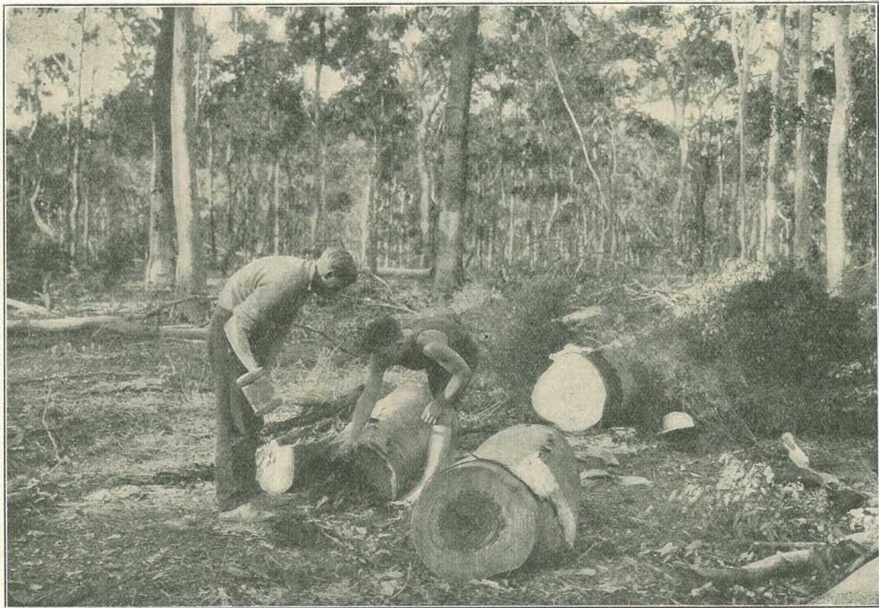
PLATE 109.—ENTERING A WEDGE. St. Lucia Trainees engaged in splitting fencing timber.
