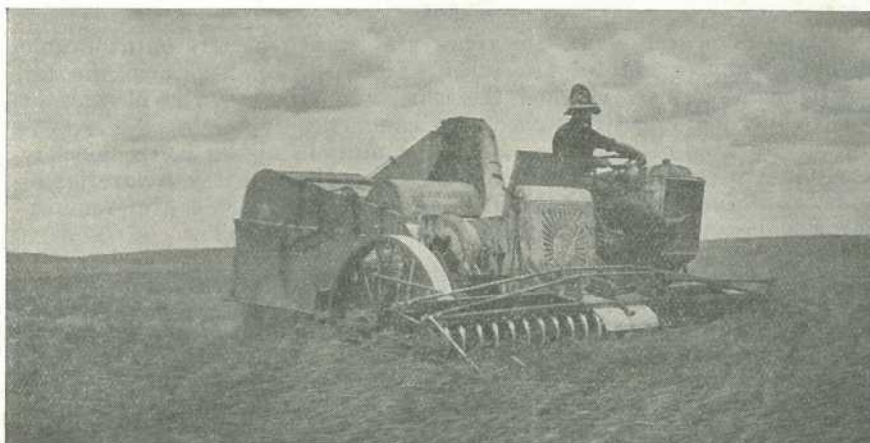
PLATE 88.—AUTO-HEADER AT WORK IN BADLY LODGED CROP, J. FLEGLER'S FARM, EVANSLEA, DARLING DOWNS.
