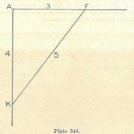
The 3-4-5 Method of Laying Out a Right Angle.
