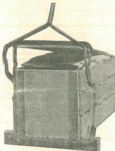
Plate 88. ANOTHER TYPE OF IRON CLAMP SHOWING CLAMP READY TO APPLY THE PRESSURE TO THE LID.
