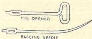
Home-made needles can be made as shown here—this particular one being made from an ordinary sardine tin opener.
