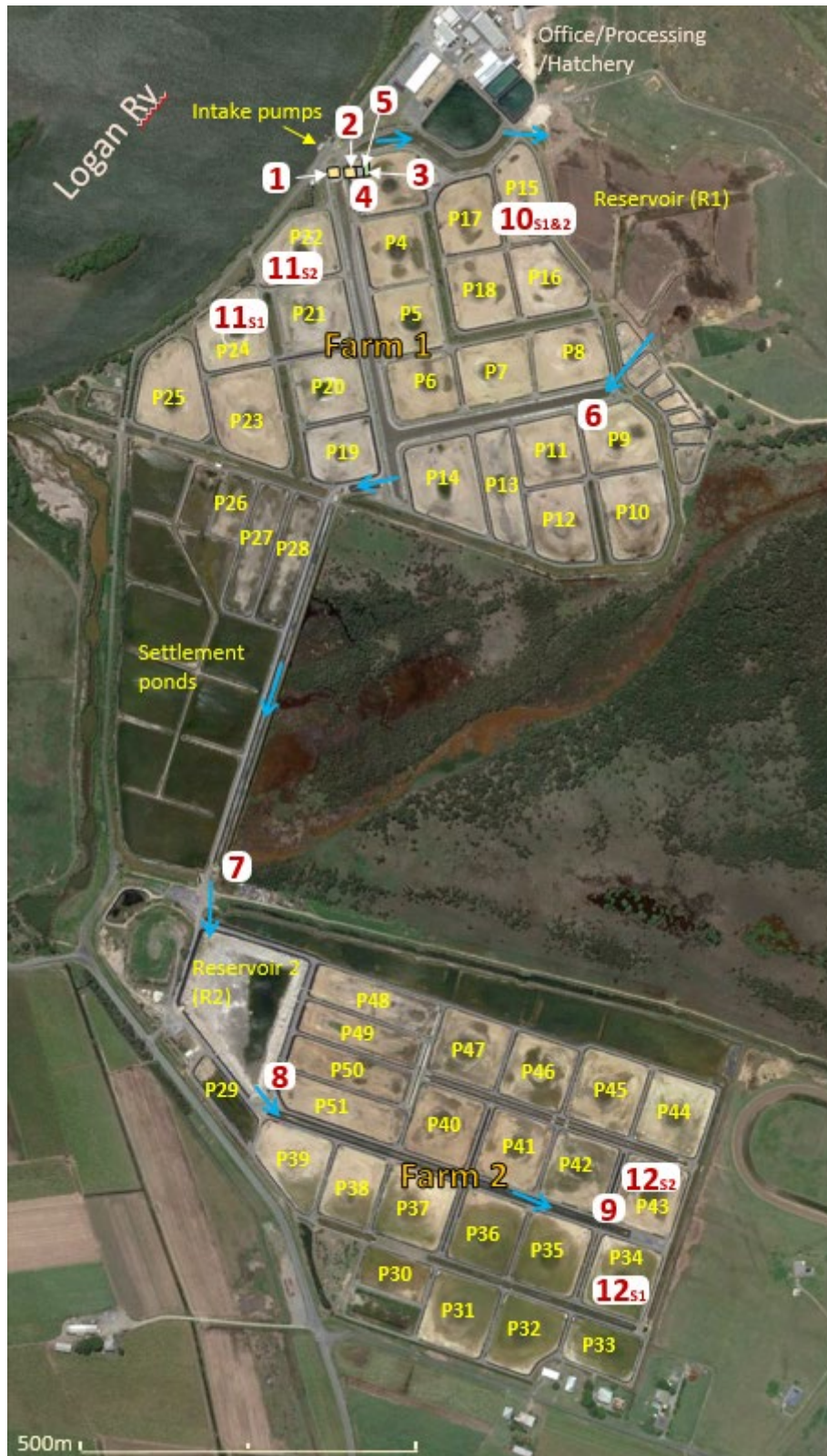
Figure 6. Layout of the GCMA farm indicating the locations of sampling points (1 to 12) and water supply flow (Blue arrows). Note that some farm features have changed since this aerial photograph was taken. S1 and S2 denote production ponds sampled in Season 1 and Season 2 respectively. Farm 1 and Farm 2, as they are generally referred to, indicate old and new sections of the same farm. See Table 3 for description of sampling points.
