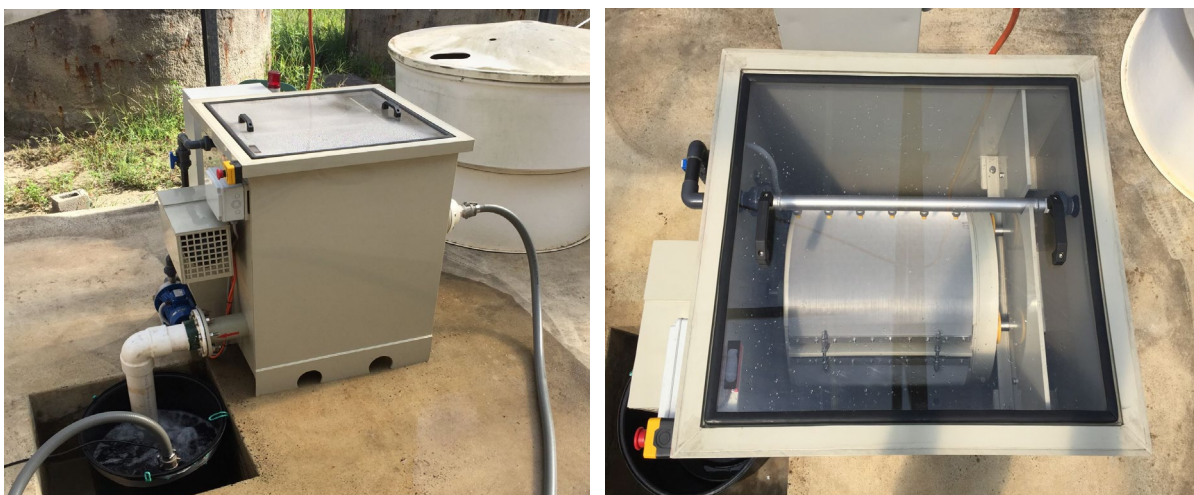
Figure 4. Rotating drum filter used for filtration experiments. The side view in the left image shows the raw water supply entering on the right of the RDF at the centre of the drum and filtrate flows into a sump below filter level. The right image is looking down on the filter drum with stainless steel mesh in place.
