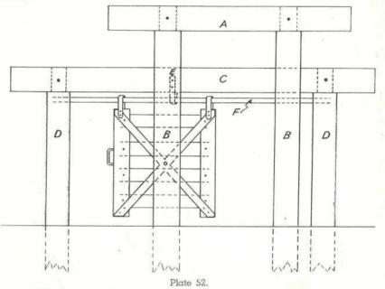
Slide Gate in Half-open Position.—When the gate is closed it is prevented from swinging by the two sets of crush posts. A, crush cap; B, crush posts; C, sliding gate cap; D, sliding gate supports; E, centre support for slide rod, hidden by post; F,  $l_{4}^{1}$  in. mild steel rod or 2 in. galvanised piping.
