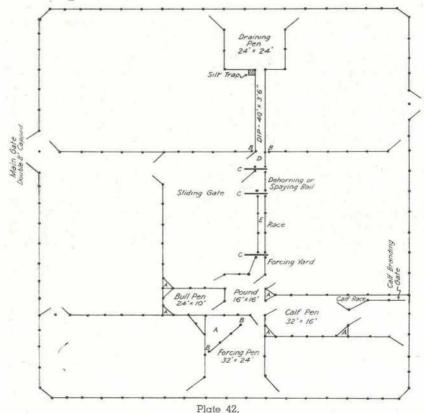
**Plan of Cattle Drafting Yards.**—A, corners for shade trees; B, spaces for slipping through when working yard; C, slide gates; D, cemented apron; E, race or crush 22–24 in. wide. Panels are 8 ft. and 6 ft., as shown by the dots, which represent posts.
