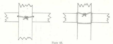
Method of Tying Rails Let in Flush With the Inside Face of the Post.— Left, rail bored; right, rail not bored.
