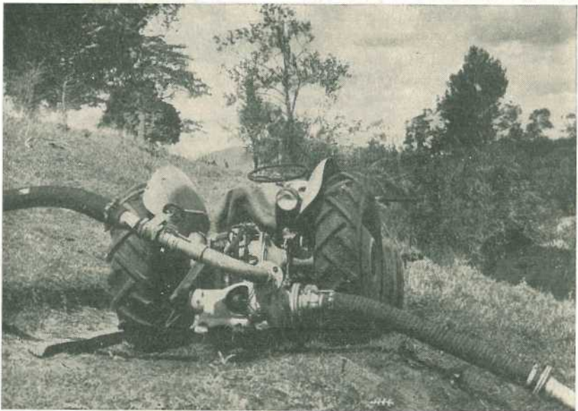
A directly mounted irrigation pump saves time and removes valuable equipment from flood risk.
