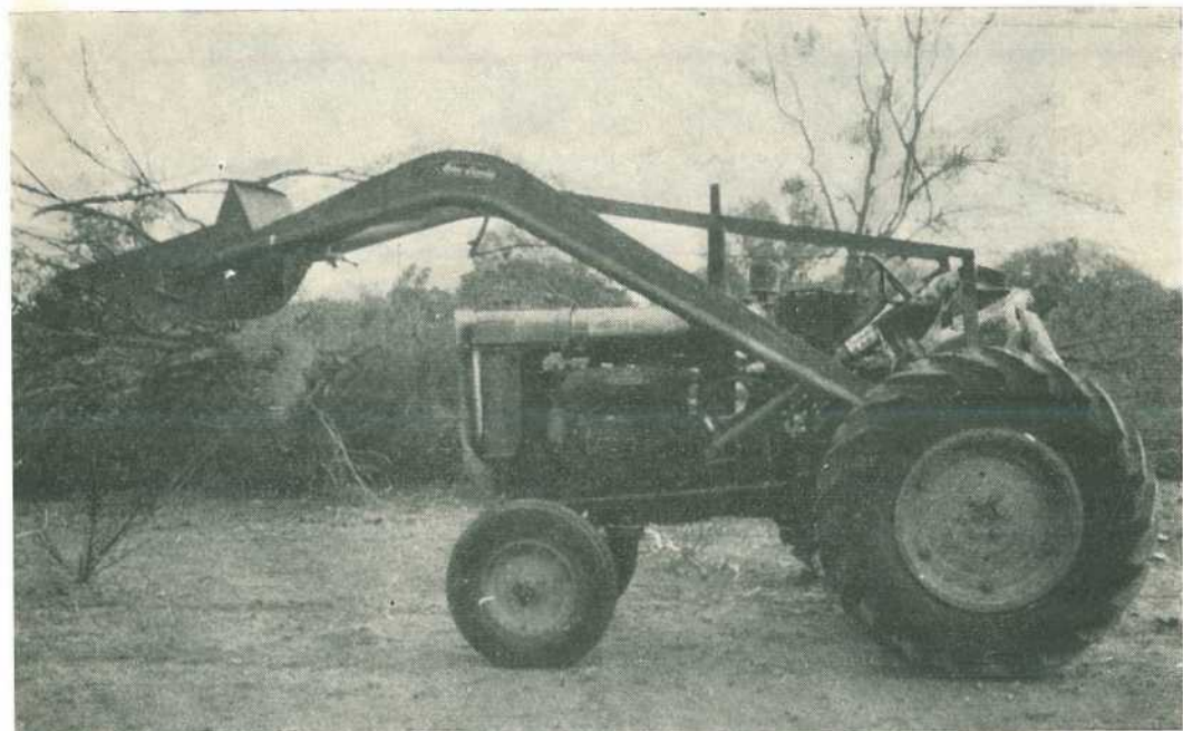
Plate 1: Fordson Diesel Mounted with Front-End Loader.
