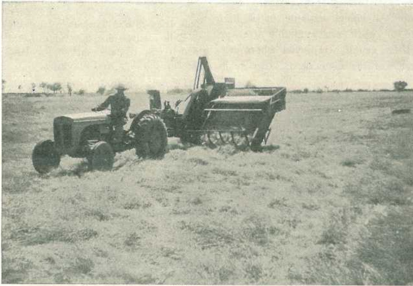
Plate 20. Tractor and Engine-functioned Hay Baler Baling Bush Hay at Colwell Station, McKinlay.
