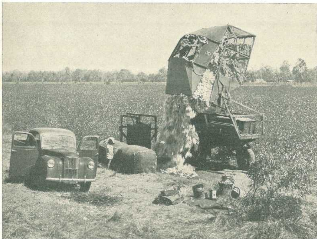
Plate 1: Machine Harvester tipping Basket of Cotton for Baling. A. W. Brownlie's irrigated property at Theodore.
