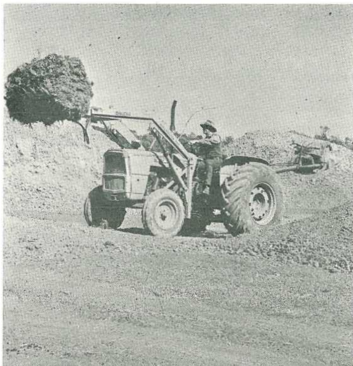
A tractor and silage grab can unload a tonne of silage from a pit in less than 10 minutes. Note counterweight at rear.
