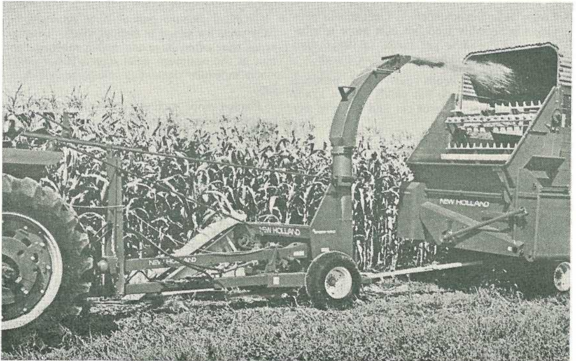
A precision chop harvester at work in a maize crop. This machine can make chopped hay as well as silage.
